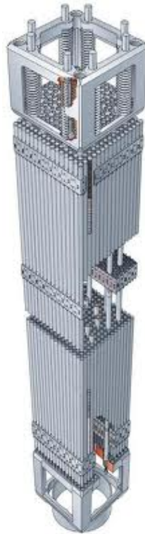
Figure 1.3: Schematic view of fuel rod element
