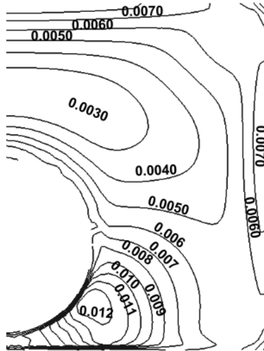
Figure 6.7: Contours of time-averaged dimensionless turbulence kinetic energy ( k/U_b^2 )
