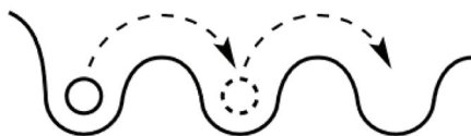
Figure 5.7: Ion hopping between sites when the thermal energy and applied AC frequency conditions are met. This process is represented by the C in the (RC) circuit. Image adapted from Ref. [25]
