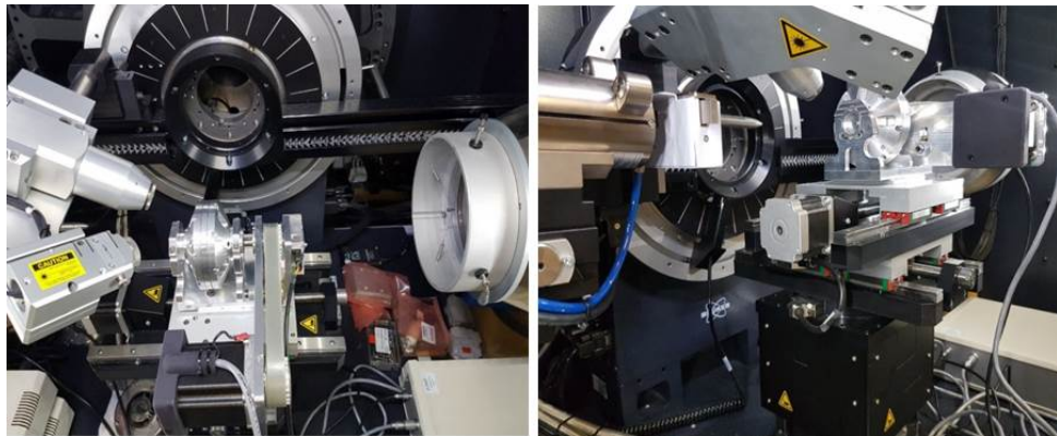
Figure 3.12: An image of the developed Couette shear cell mounted at the lab-scale X-ray diffractometer Bruker D8-Discover
