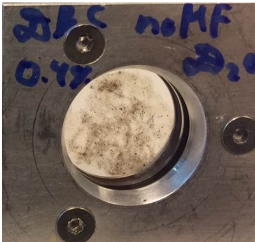
Figure 5.1: Photo of the deuterated bacterial cellulose suspension filled in the experimental cell for SANS measurements.
