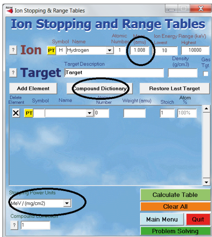
Figure C.3 SRIM input window. Add your elements or compounds. Be sure to use: the correct density, weight of the particle and units [keV/micron].
