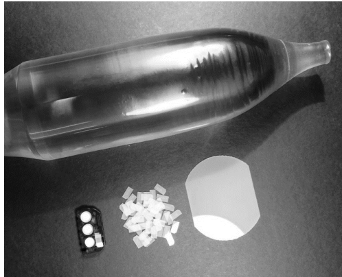
Figure 2-1: Al_2O_3:C,Mg single crystal (top), polished wafer (bottom right), FNTDs (bottom middle) and OSL slide with FNTD chip covered by three converters (polyethylene, Teflon and Li-glass) (bottom left).
