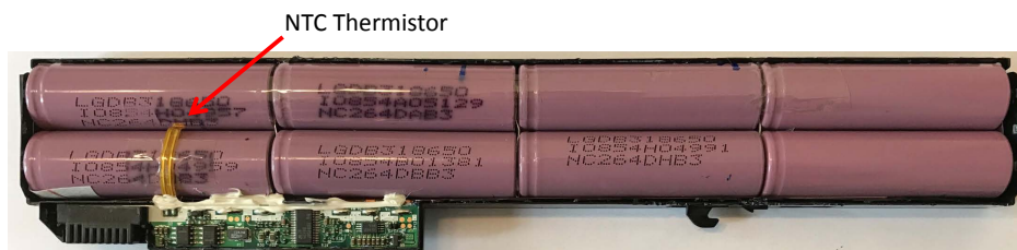
Fig. 3.2: Example of a 73 Wh laptop battery pack with 10 k \Omega NTC thermistor. Note that a piece of tape is normally present to fix the thermistor onto the batteries but this was removed for clarity.
