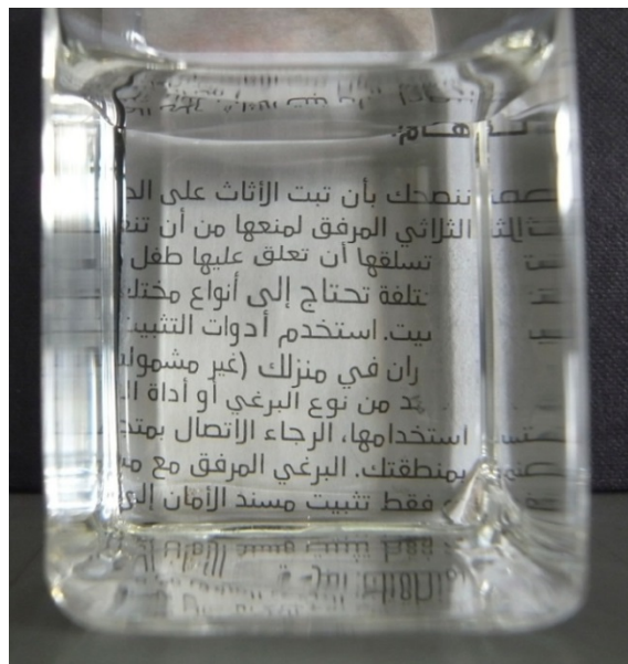
Figure 7.1. A photograph in daylight of a 40x40 mm 2 square cell containing an RFG gel which had been irradiated with two, 10 mm diameter crossed X-ray beams each with an average dose of ~20 Gy. For a fluorescent image of the same gel see figure 7.8.
