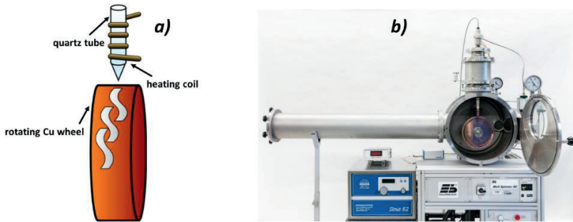
Figure 3.2: a) Schematic drawing of the melt spinning, b) melt spinner (Edmund Bühler GmbH) [3].
