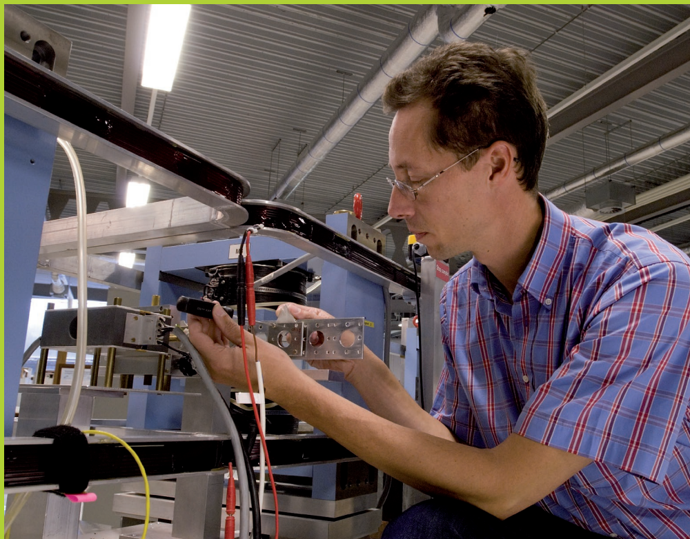
Figure 7: The sample position of the SESANS instrument.
