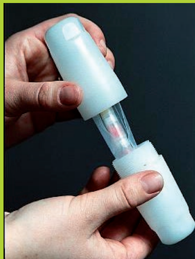
Figure 9: Polyethylene (PE) "rabbits" in which four strings of plastic-packaged (PE) sample-capsules. Each string contains four samples with neutron flux monitors, adding up to 16 samples per PE rabbit, irradiated together in a pneumatically operated irradiation facility
