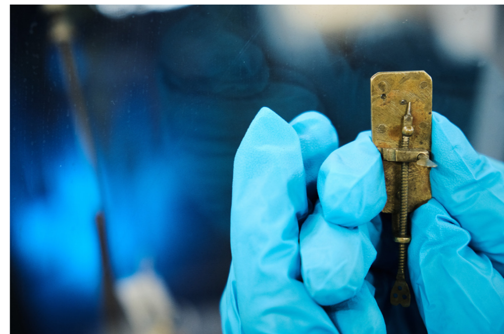
Photo: This original microscope was brought to the RID for inspection at FISH. Antonie van Leeuwenhoek would place the specimen for investigation on the tiny pin which he would then align in front of the lens (behind the centre hole in the brass plate).
