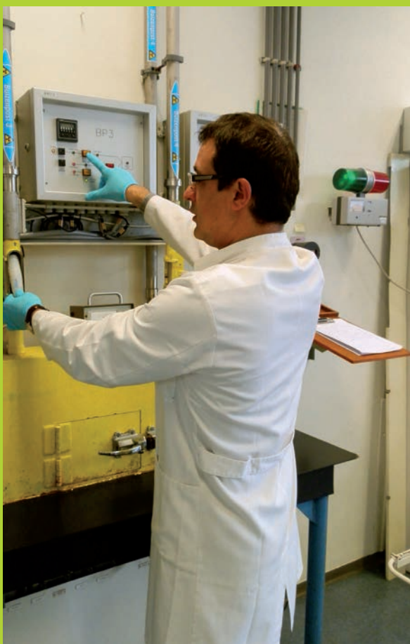
Pneumatically operated small-target irradiation facilities. The photograph shows the PE rabbit loaded into the inlet of the pneumatically operated transport system (to and from the irradiation position).
