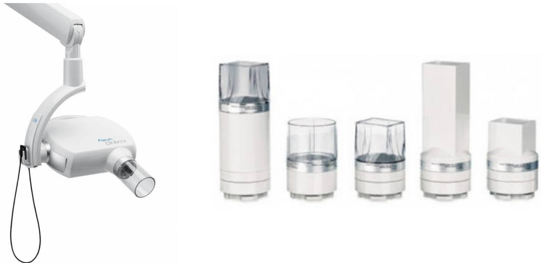
Figure 2: left: an X-ray machine for dental applications, right: different spacer shapes, with a long and short spacer cone and round and square collimators. A spacer limits the beam size and ensures a constant focus to skin distance.
