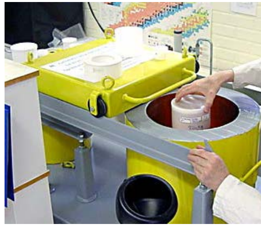
Figure 4.2. Marinelli beaker is placed on the Ge-detector in the lead castle
