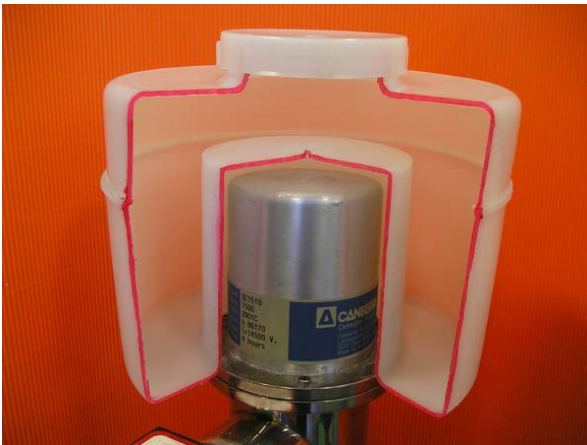
Figure 4.1. Cross-section Marinelli beaker
