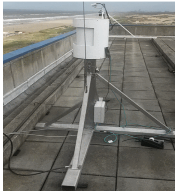
The RiegI VZ2000 scanner permanently at work in Kijkduin
