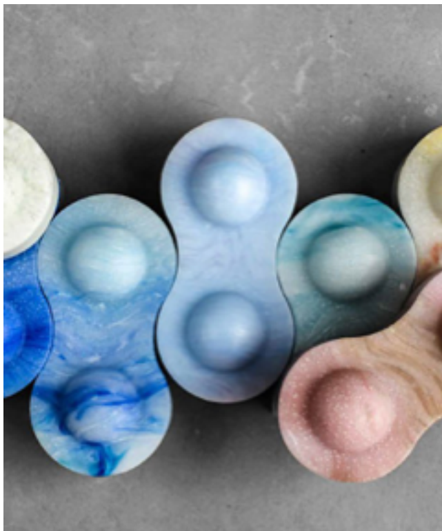
Fig. 10 Prototypes of recyclable, reducible and reusable cast glass components, developed at the Glass Lab for the R3 Glass project
