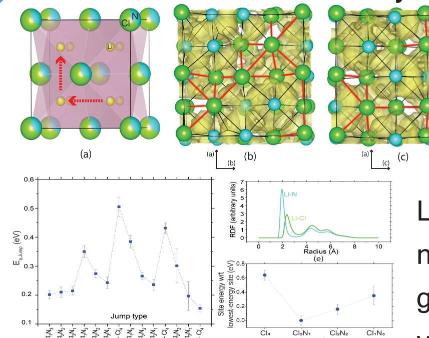
Molecular dynamics in solid electrolytes is a key technique to grasp the diffusion mechanisms. For example in Li<sub>5</sub>NCl<sub>2</sub>, one of the few compositions that is stable against
