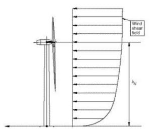
Figure 1: Horizontal Axis Wind Turbine operating in shear flow
