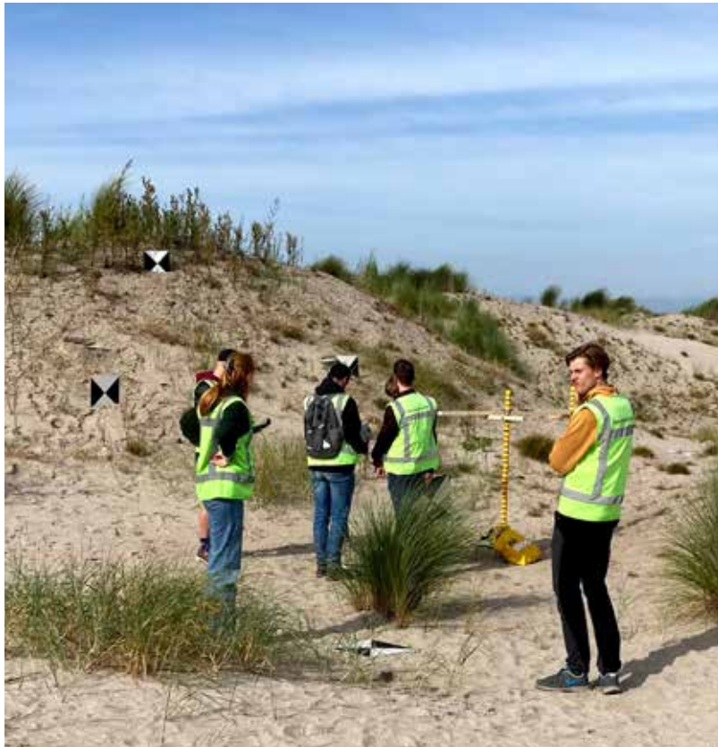
With cameras on the screw piles, a 3D image is made of the dune using stereo vision.
