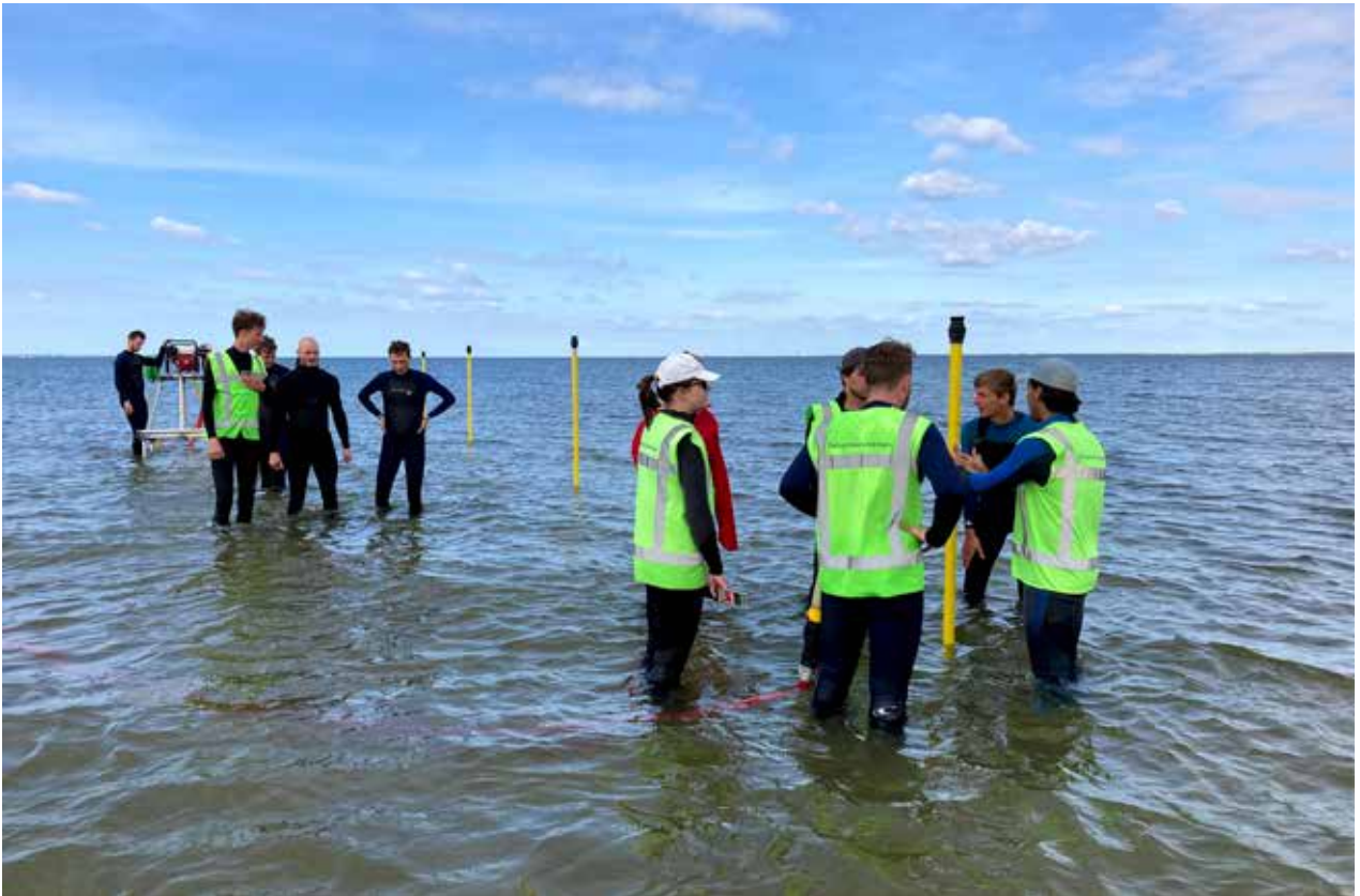
The installation of jet poles. The acoustic doppler velocimeter will be placed on the poles to accurately determine the flow speed and wave direction in the surf. (Photos supplied by Anne Ton)
