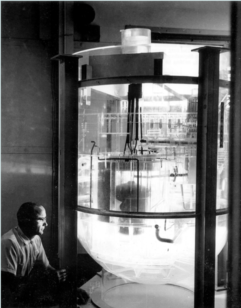
One-sixth scale model of Oak Ridge National Laboratory's Molten Salt Reactor Experiment. The MSRE achieved criticality June 1, 1965, and reached its full power of 7,500 kilowatts in May 1966. c. 1968 (Photo: US Department of Energy)
