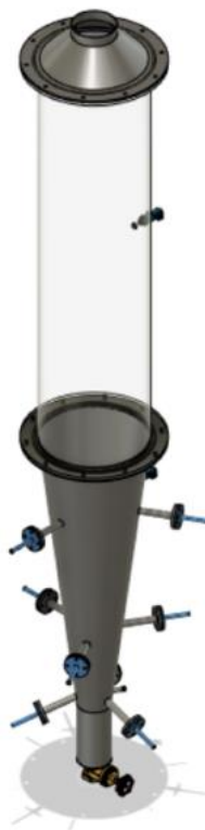
Figure 1. Design - Cold fluidized bed setup [1]
