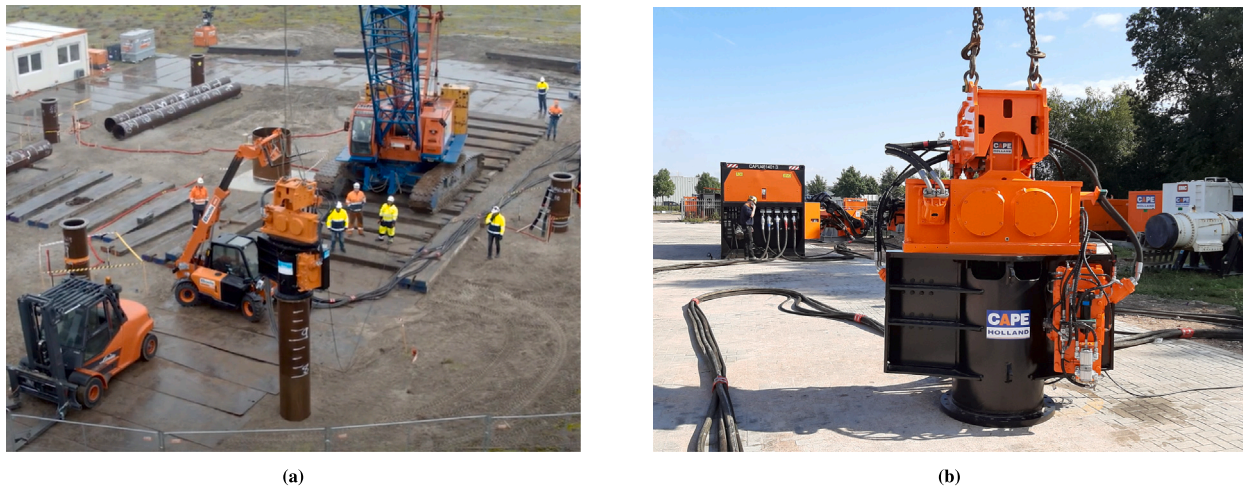
Fig. 1. (a) The test site of the GDP field campaign and (b) the GDP shaker at the manufacturing site.
