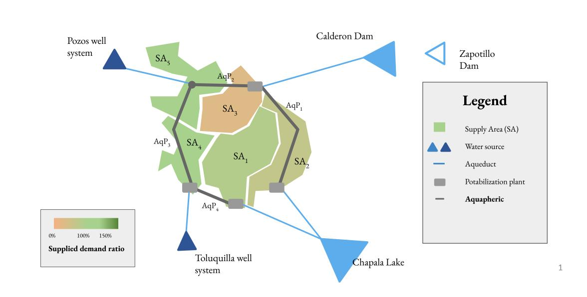
In response to this vulnerability, in 2022, the Government built the **Aquapheric** (AqP): a circular aqueduct that interconnects the five supply areas and can pump up to **1 m3/s** of water in both directions in each of its four segments independently. This infrastructure can significantly increase the city's resilience to drought, however, an operation policy has not yet been made.
