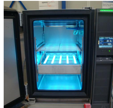
Fig. 2: Climate chamber with UV light [5].
