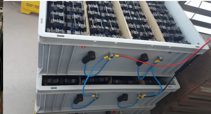
2 X 12V Sea Salt Batteries in Parallel ca. 400Wh 40Ah
