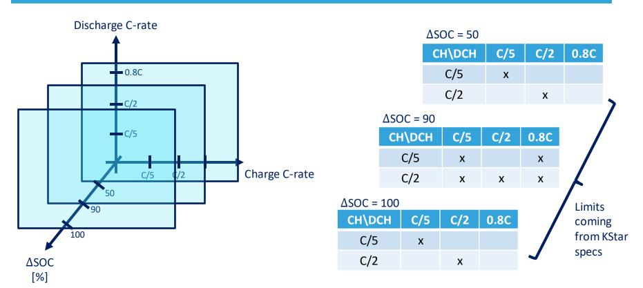
Each test has 2 cells and 2 types of experiments (characterization & cycling)
