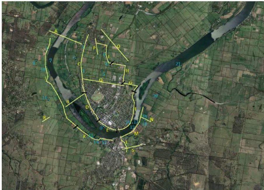
Figure G.48: Output locations for water level (blue) and discharge (yellow) around Grafton.
