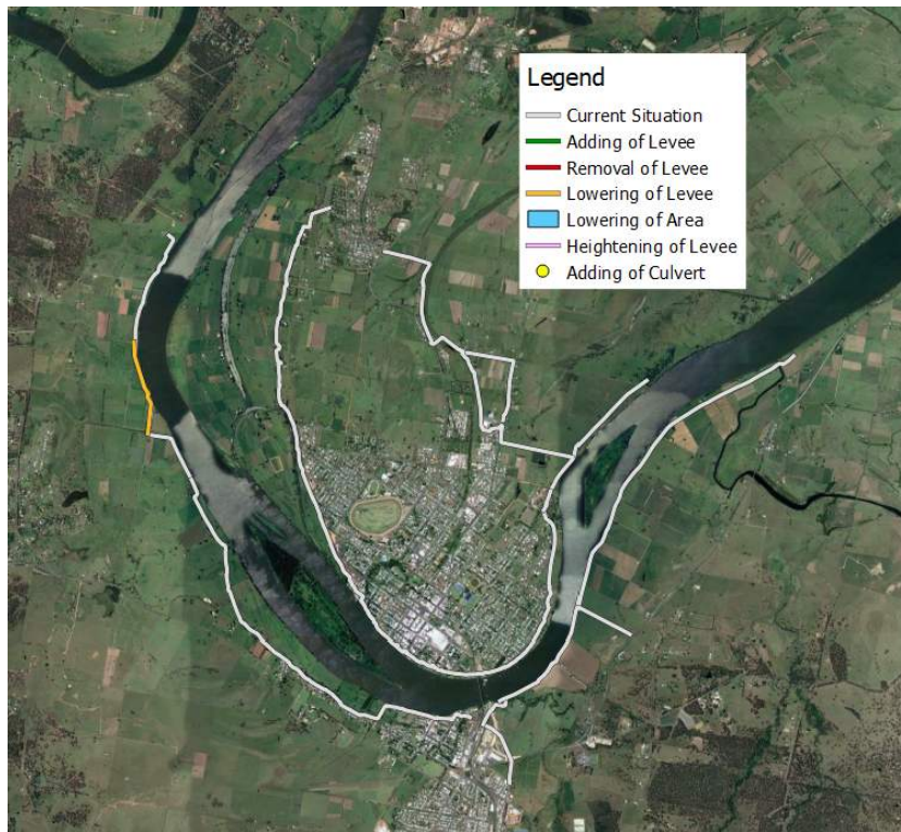
Figure F.4: Scenario 2.1: Lowering Waterview Levee (upstream).
