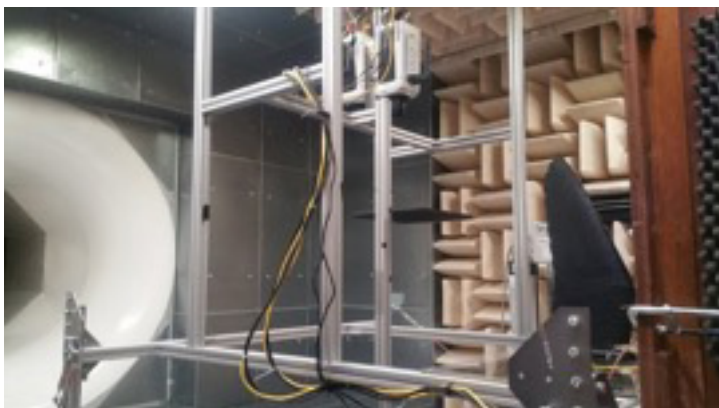
Model wing of robotic bird in windtunnel setup for PIV measurements. White arrow indicates wing in vertical position. Flow direction from right to left.
