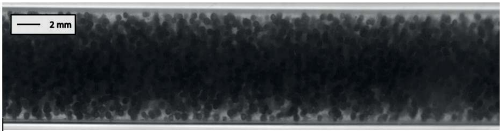
Figure 1 : Snapshot of a densely laden pipe flow with a particle concentration of 22.5%, captured with optical imaging.
