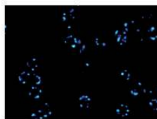
a) SiO 2 raspberry particles. b) Raspberry particles imaged by CSLM
