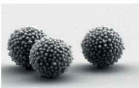
a) SiO 2 raspberry particles. b) Raspberry particles imaged by CSLM
