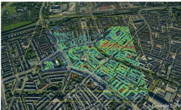
The mapping of pollution by iso-lines: concentration contours of O 3 (indicating locations with enhanced ozone distribution as result of the chemical reactions) – in the horizontal plane at pedestrian level (z=2 m). Results of the integrated in-house developed CFD/CRD solver for the photochemical smog generation for a city of Rotterdam, Liu and Kenjeres (2017)
