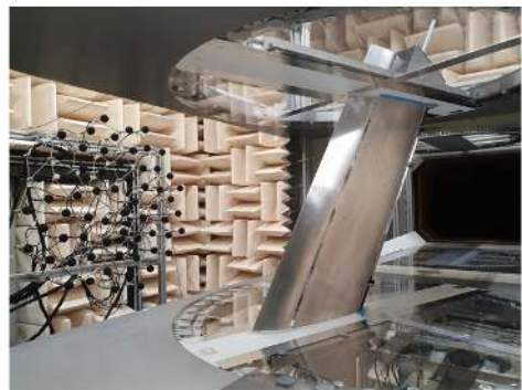
Experimental setup at the University of Twente with the high-lift device in swept wing configuration
