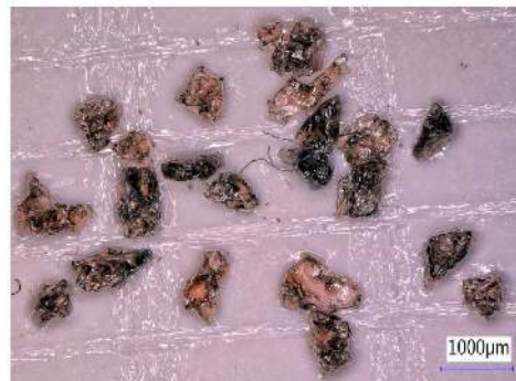
Top view of the grit particles placed on the flat plate surface.
