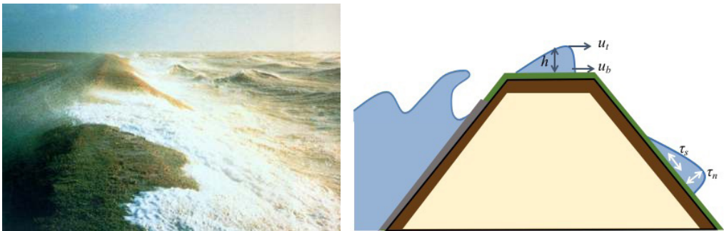
Figure 1: Waves approach the dike and break on the seaward dike slope. The broken waves run up the dike, overtop the crest and then run down along the landward slope. Left: photograph of grass covered dike during wave overtopping [5] (Picture courtesy: HR Wallingford). Right: Schematization of wave overtopping on a grass-covered dike. The overtopping flow has a layer thickness h , the flow velocity near the bed u_b and the flow velocity in the top layer u_t . Typical layer thickness and velocities range between 1-50 cm and 1-10 m/s respective. The waves pull on the grass cover with a shear stress \tau_s parallel to the dike surface and a normal stress \tau_n perpendicular to the dike surface (figure adapter after [4]).
