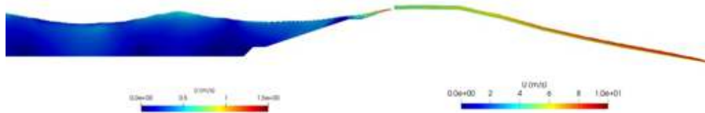
Figure 3: Numerical simulation of waves running up the dike with a berm and cause wave overtopping (Left). Overtopping waves run over the crest and cause high shear and normal forces due to the high velocities and turbulence (Right).
