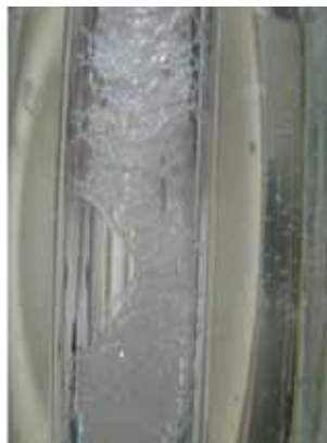
Foam from an experiment with 2000 ppm V-502 foamer and 50% heptane. The left picture is taken at the beginning and the right a picture is taken at the end of the experiment.
