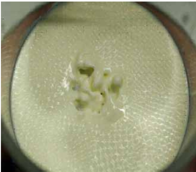
Formation of persistent holes and finger like protrusions in thin layers of cornstarch that are shaken at high accelerations.
