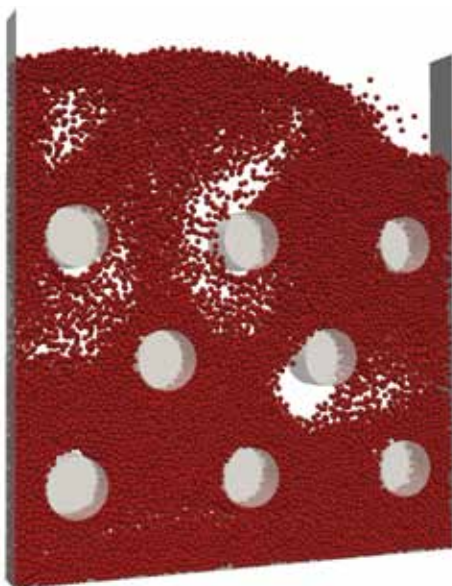
Snapshot of eight immersed membrane tubes in a DPM simulation
