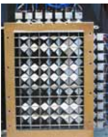
Left: A photograph of the active grid. (a) energy input in turbulence as a function of the ratio of integral time scales of windtunnel turbulence and GOY model random numbers, shown for different shell truncations of the GOY velocity field. (b) Anisotropy of wind-tunnel turbulence
