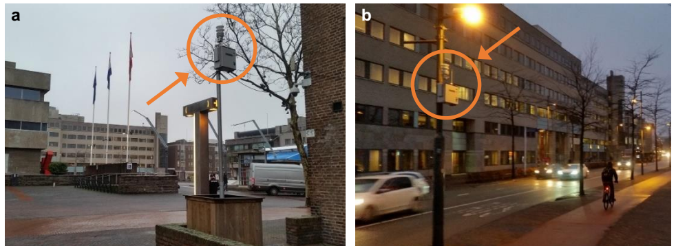
Photographs of 2 (out of 10) monitoring stations (Grimm 164DM spectrometer + Luft WS500 weather sensor) as adopted in the measurement campaign in the city centre of Eindhoven.
