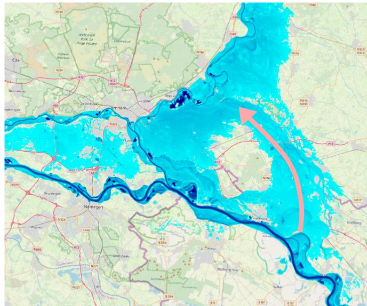
Figure 5: Dike breaches in Germany may result in significant overland flow (pink arrow) resulting in inundations of the Dutch hinterland influencing Dutch flood risk.
