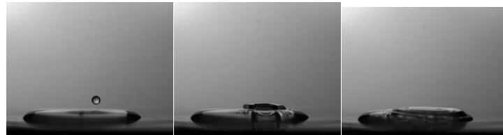
Image sequence of a droplet impacting the substrate at low pressure conditions
