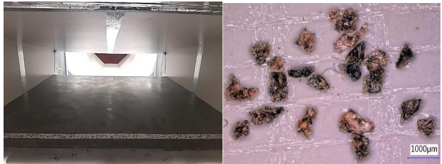
Left: Flat plate with the grits elements distributed near the leading edge. Right: Top view of the grit particles placed on the flat plate surface
