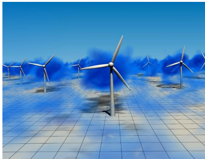
Visualization of the low speed wind regions, known as wind turbine wakes, in a very large wind farm. The intensity of blue cloud indicates the strength of the wind turbine wakes. Visualization by Srinidhi N. Gadde.
