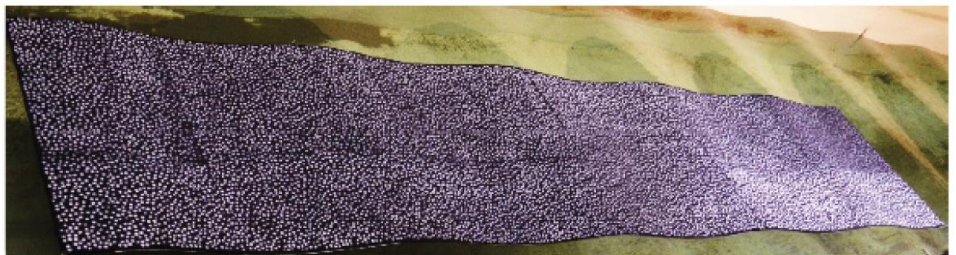
Model of VFFS with speckle pattern for DIC measurements in the towing tank of TU Delft. Wave propagating from right to left
