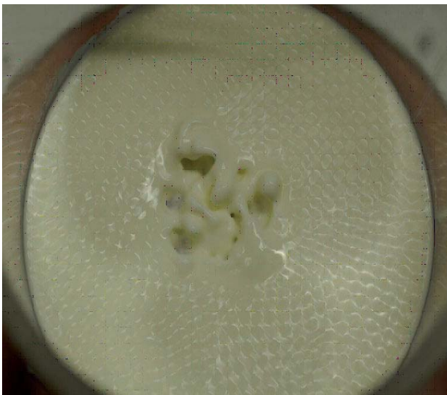
Formation of persistent holes and finger like protrusions in thin layers of cornstarch that are shaken at high accelerations.
