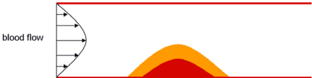
Schematic representation of the modeling of blood flow and blood clot formation. The inner part of the clot will be modeled as a poro-(visco)-elastic solid (red) and the outer layer will be modeled as a porous fluid (yellow).
