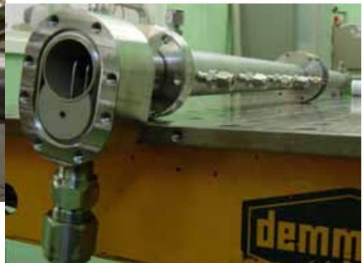
Optically accessible test section with central heating rod (left) and the entire annulus required to fully develop the flow before the Freon enters the test section (right)
