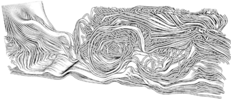
Visualization of a simulated thermally-driven turbulent flow using a depth-dependent halo technique (selected by the American Physical Society for the Gallery of Fluid Motion, November 2011)
