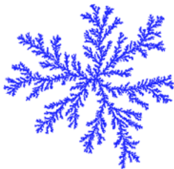
Example of a simulation result of 2D Diffusion Limited Aggregation with 10 6 particles
