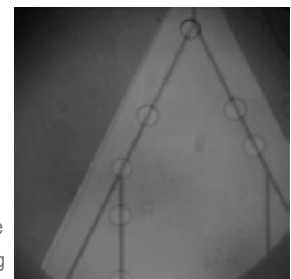
Measurement of drops inside a microchannel being guided over the gap between electrodes by applying a voltage over the gap.
