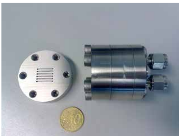
SS microreactor module without membrane integration, made for ATR tests (TU/e)
