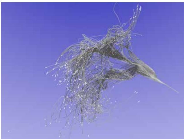
A sketch illustrating the dispersion of a bunch of tracers released from a point wise source and dispersing in a homogenous and isotropic velocity field.
