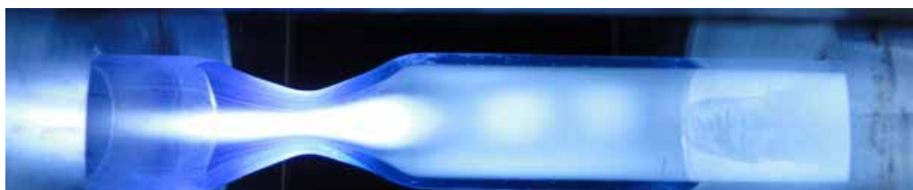
A picture of a flowing microwave-induced plasma in CO 2 . Taken from: http://differ.nl .
