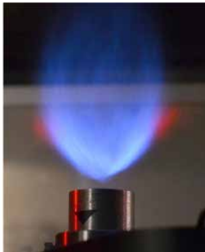
Exploded view and actual photo of a low-swirl burner with a fractal grid installed.
