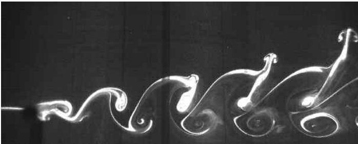
Figure 1 Side-view visualization of the flow around a heated cylinder for Re = 117 and Ri = 1 [2]. The flow is from left to right, the cylinder is positioned at the left.
