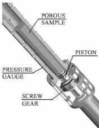
Figure 1 Experimental set-up. The screw gear unit allows adjustment for a of the porous sample with respect Bentheim sandstone.
