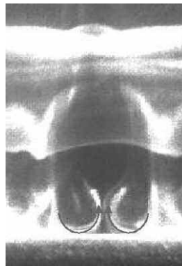
Figure 2-3 Top-view of the vortex shedding process for Re = 117 and Ri = 1 [2]. The flow is from bottom to top, the cylinder is positioned at the bottom. Left: escape of mushroom-type structures, right: a detail of the flow at the rear end of the cylinder showing a pair of counter-rotating vortices.
