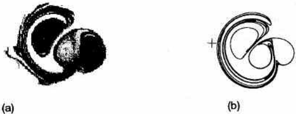
Figure 2 (a) Plan-view of the experimental tripolar vortex (dye visualization) and (b) the numerical contour-kinematics simulation with three modulated point vortices.
