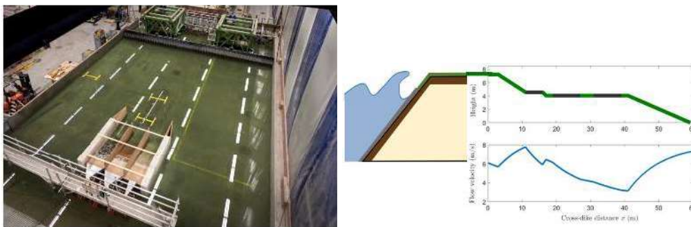
Figure 2: Left: Flume experiments in the Pacific Basin at Deltares to quantify the effect of a berm and revetments on overtopping discharge [3] (Picture courtesy W. Chen). Right: Results of the analytical model [7] to simulate flow velocity and layer thickness along a complex landward slope [1].
