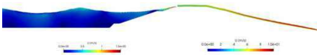
Figure 3: Numerical simulation of waves running up the dike with a berm and cause wave overtopping (Left). Overtopping waves run over the crest and cause high shear and normal forces due to the high velocities and turbulence (Right).
