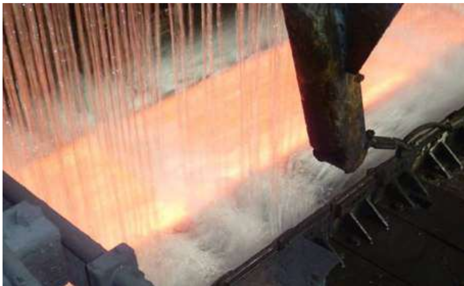
Figure 1: Run Out Table: Multiple water jets impinging on the moving, red hot, steel slab.
