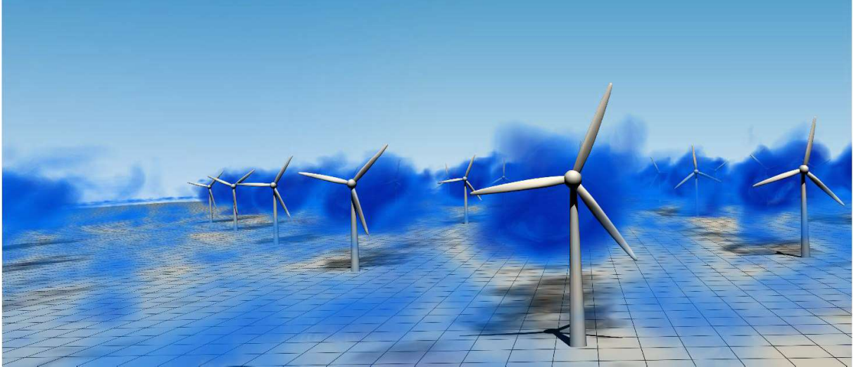
Figure 1: Flow visualization of turbine wakes from a large eddy simulation of a wind farm. Wind turbines extract energy from the incoming wind and produce a low-speed wake (blue smoke in the figure). Figure adapted from Gadde (2021) [1].
