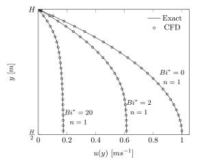
**Fig. 5:** Velocity profiles obtained with ReFRESCO and exact solution for different  $Bn^*$ . The duct has L = 20H and was discretized with a grid 640x96.
