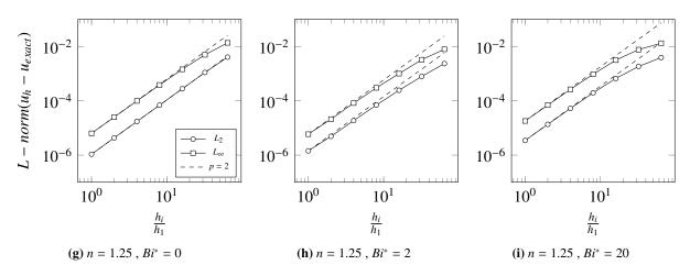
**Fig. 6:**  $L_2$  and  $L_{\infty}$  norm of the discretization error of the velocity for different combinations of  $Bi^*$  and n.  $u_h$  is the solution computed on the grid h.
