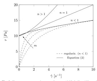
**Fig. 2:** Shear stress versus shear rate for  $\tau_0 = 10 [Pa]$ ,  $K = 1[Pa \cdot s^n]$  and different values of the flow index *n*. The Papanastasiou regularization is plotted varying the parameter *m*.
