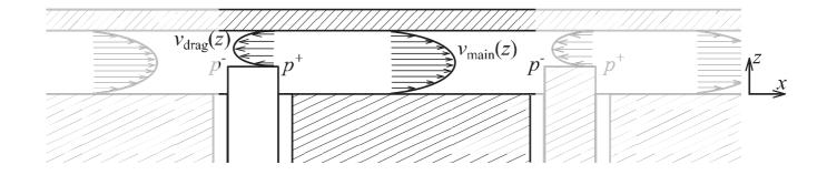
1 Basic principle of the contactless actuator, with the larger flow to the right creating a net viscous force on the substrate above.
