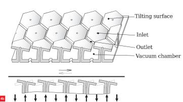
In this demonstrator a wafer was placed on top of the manufactured actuator. With a pressure controller a steady fly height of 15 µm was achieved. For a video demonstration of this system see [3] and [4].
