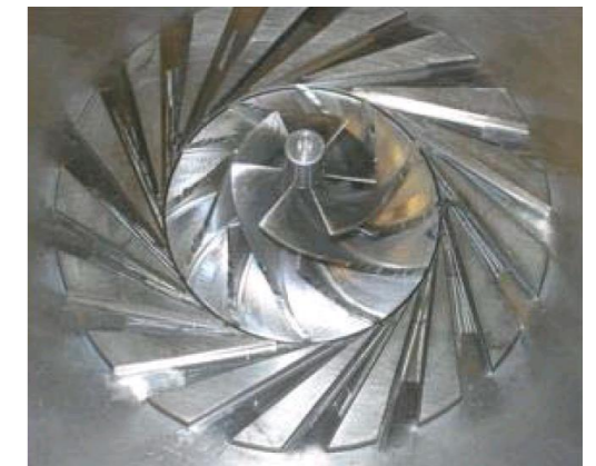
Part drawing and photograph of the SNL main compressor [3]
