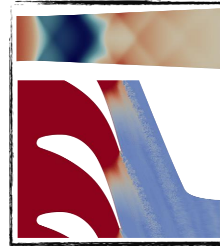
CONDENSING WET STEAM (LES) [5]
