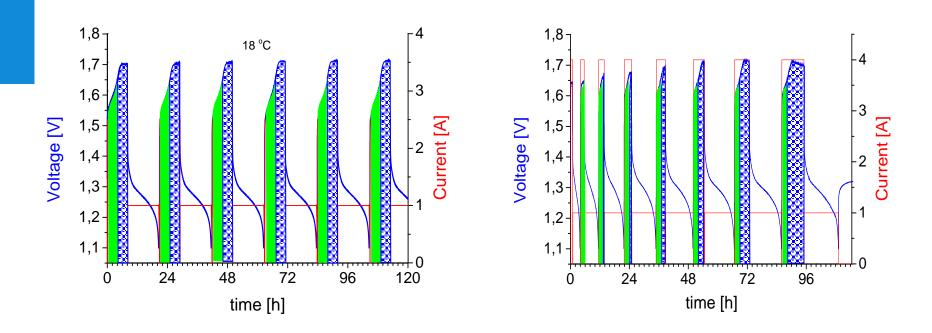
Current: applied currents during charge, electrolysis, and discharge Voltage: that is the voltage that results when using these currents Several cycles with constant (left) or increasing (right) current insertion.
