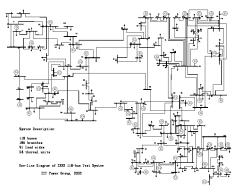
■ 54 thermal units; 118 buses; 186 transmission lines; 91 loads
