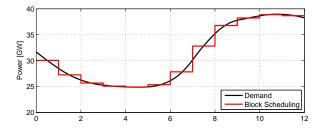
Generators try to follow the stepwise energy profile Generation-Demand balance is needed in real time
