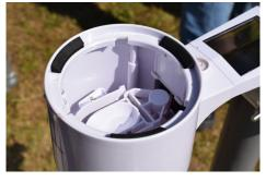
Figure 1: Tipping bucket mechanisms.
