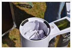
(b) Testing of tipping bucket mechanism
