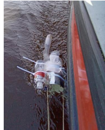
Figure 2. Towing a constructed mini-trawl through the water by boat.
