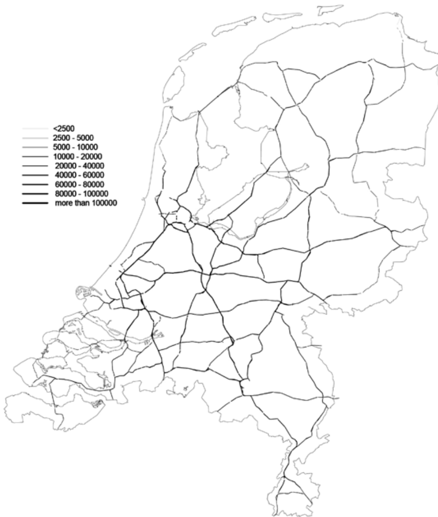
Figure 16.2 Example of an intensity forecast in vehicles per day for 2021, in The Netherlands
