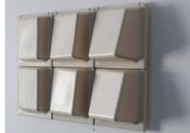
Stoneware slipcast prototype showing competent level morphology changes. Credit: Jason Volken, Kelly Winn, CASE.
