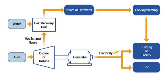
Figure 3.3.: Diagram of a CHP Installation [10]
