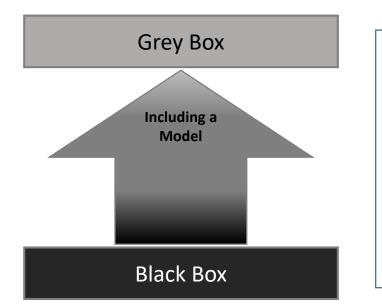
When **data-driven models** (black box models) are (partly) supported by **explicit models** (equations) with a physical meaning
