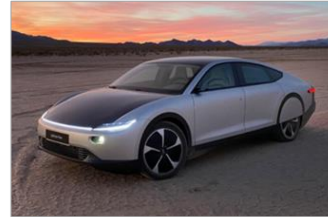
3D-shaped system with high-efficiency silicon cells (4,5 m 2 ) on Lightyear One
